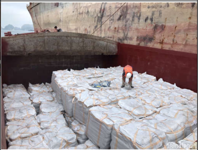
Increment samples were taken randomly during loading
